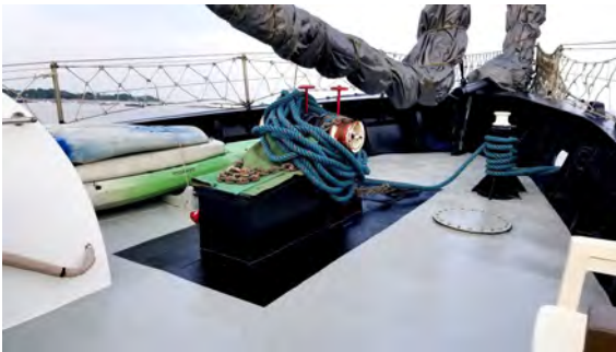
The photo at the left shows the forecastle finished with all welding repairs done and completely repainted. This work is continuing now in the midship area where we are cutting away some rusted plating and welding in the new. Painting will follow within a few days.
